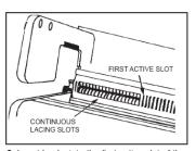
3. Insert hooks into the first active slot of the face strip. Secure with lacer pin.
