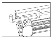
2. Position lacer head to the end of the tool. Turn knob clockwise to open rollers.
