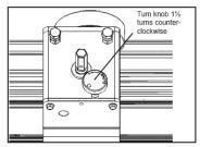
5. Return lacer head to end of lacer and turn adjusting knob 11/2 additional turns counterclockwise.
