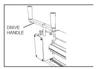
6. Using the handle, move the lacer head acros the belt width at a smooth speed.
